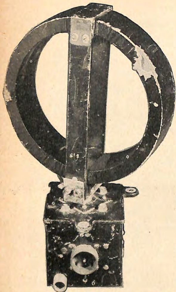
Figure 356. Radio Homing and D/F loop antenna used with some types of Japanese airborne equipment.
